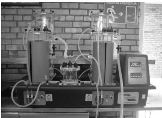
Figura 1. Digestor anaerobio ARMFIELD W8
