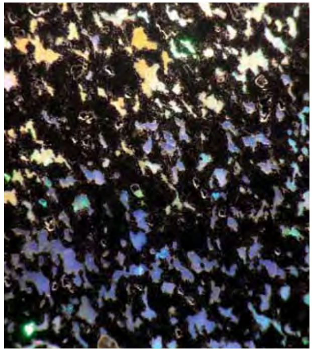
Figure 10. This detail from the 205 ct polished sample in figure 9 displays oriented (bottom right to top left) irregularly shaped vesicles filled with opal that varies in bodycolor from blue (bottom) to yellow, pink, and white (top). Photo by Graham Henry; field of view is 18 mm high.
